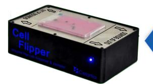
Put incubated **Petaka ET** on top of the powered Cell Flipper platform and allow the gliders to oscil[ate randomly for 30 sec. to 1 minute
